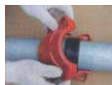
3. Fitting Assembly: Place the housing over the gasket and insert bolts. Then tighten the nuts by hand.
