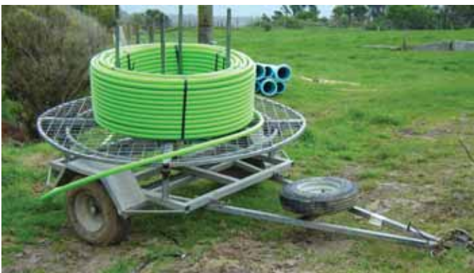
DN 32 PE telecommunication duct in a 500m coil on a coil dispensing trailer
