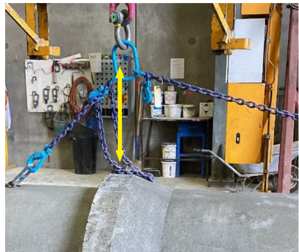
Figure 8. The top of the chain must be above the Collar side within the area where the collar's highest lip is located.
