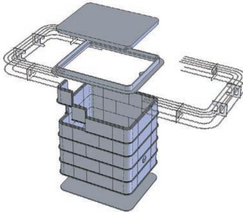
If the chamber layers are left in the sun pre-installation, expansion may occur. In this case, it is necessary to leave one section out of the layer until it is assembled onto the chamber in the ground. This will give more flexibility to ensure layers are locked together. Replace that section as each layer is completed.
