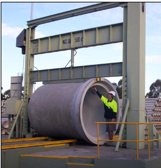
Load testing of Steel Reinforced Concrete Pipe
