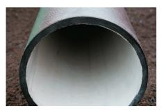
Material used in the manufacture of ductile iron is: as per AS1831:2007, ductile iron mechanical properties 450-10. Cement: as per AS/NZS 2280:2004 section 2.5.2. External coating: as per AS/NZS 2280:2004 section 2.4.1 – 2.4.2.
