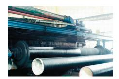
Humes ductile iron pipe is lined with ordinary Portland Cement in accordance with AS 3972. The lining is applied through centrifugal spinning of the pipe. A smooth finish and high compaction is achieved by this method, giving excellent hydraulic performance.
