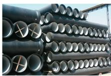
Humes ductile iron pipe is zinc coated and then painted with bituminous paint in accordance with AS/NZS 2280:2004. In low corrosive soils, this removes the need for a PE sleeve (subject to council requirements). In highly corrosive soils, Humes recommends the use of a PE sleeve fitted to the outside of the pipe to increase protection. These are available on request through Humes.
