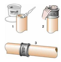
along the central axis of the pipeline. Apply a horizontal forward pressure, in combination with a small side to side movement, and push the pipe home into the sleeve coupling.
