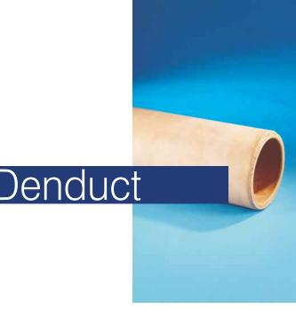
The Naylor Denduct underground duct system consists of DN100 and 150 vitrified clay plain-end ducts with flexible sleeve couplings and fittings. It is especially ideal for the enclosure and protection of underground cables or other services on heavy civil projects where the inherent strength of the ducting system is important.
