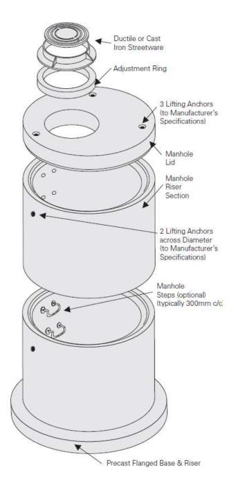
Figure 1 Schematic Diagram of Precast Manhole General arrangement
