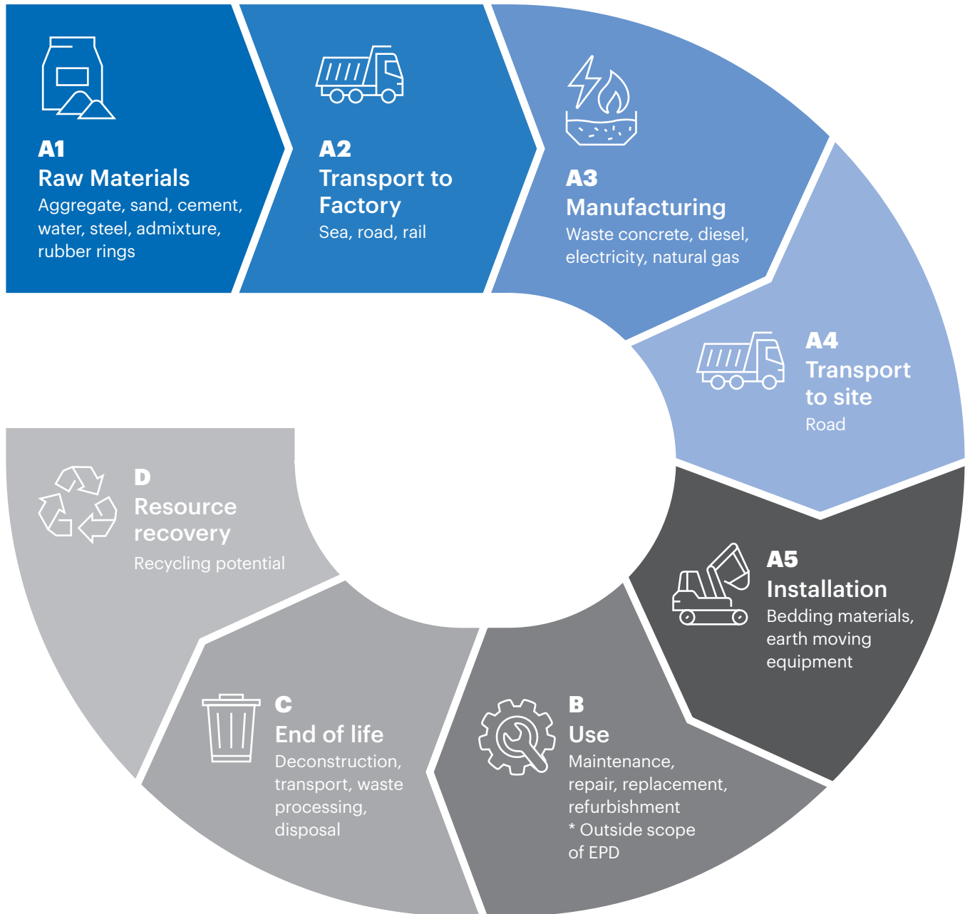
Figure 1 – Product lifecycle of steel reinforced pipes
