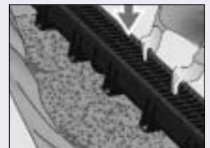
Place in trench
