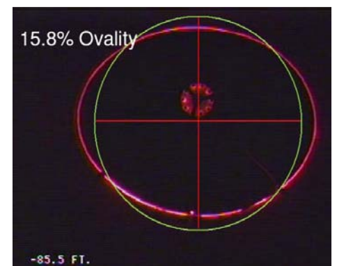
Example of the laser profile showing the deflection (red) and the original (green)
